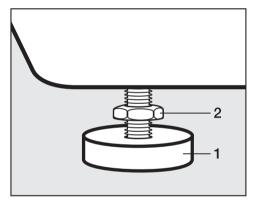
Using the spanner supplied turn counternut 2 in a clockwise direction.
